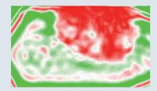
**Types of defects:** delamination and density fluctuations before and after the sintering process
